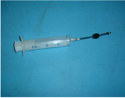
Figure 72: Syringe with Filter for Flushing
