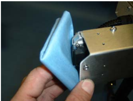
Figure 84: Hold Lint Free Wipe Up to Nozzle
