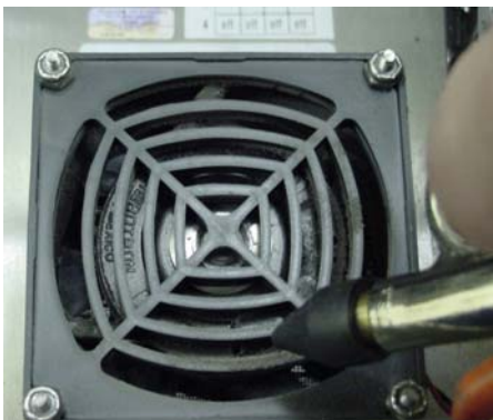
Figure 52: Blow Out Fan
