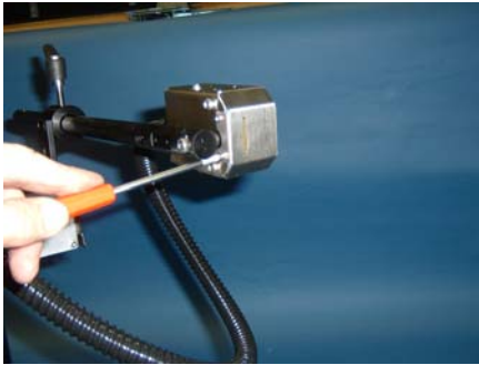
Figure 79: Loosen 128 Nozzle Plate Screws
