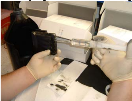
Figure 73: Flushing with Syringe
