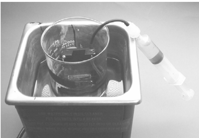
Figure 92: Cleaning a Severe Clog
