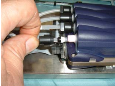
Figure 64: Remove Tubing from Printhead
