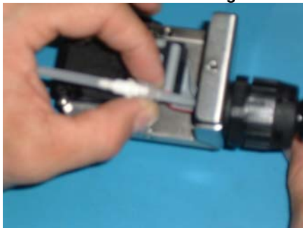
Figure 96: Disconnect Lure Fittings
