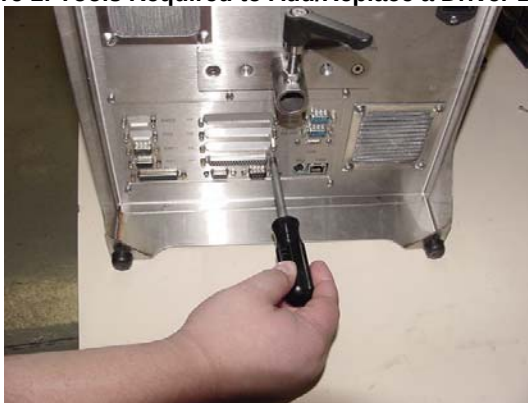
Figure 2: Removing Jack Screws
