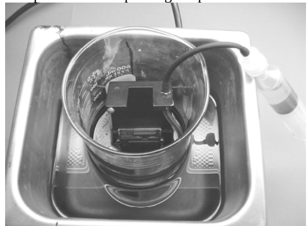
Figure 92: Cleaning a Severe Clog
