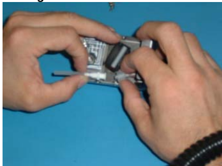
Figure 99: Re-Attach the Printhead
