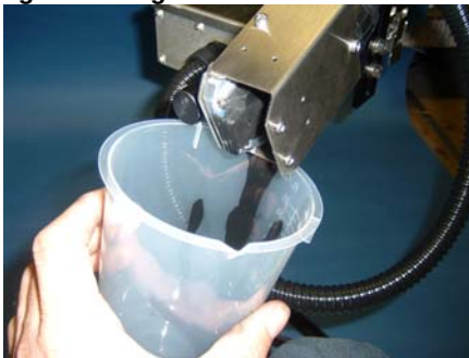
Figure 88: Priming into Container
