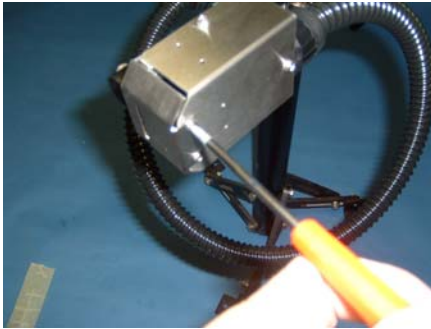
Figure 87: Tighten Nozzle Plate Screws
