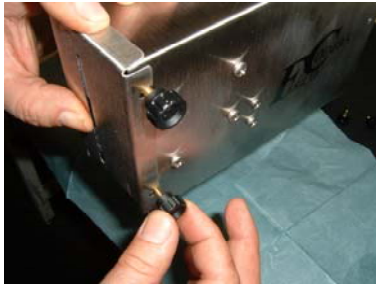
Figure 60: Loosen Thumb Screws
