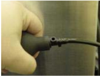
Figure 83: Pump the Priming Bulb
