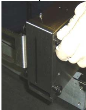
Figure 55: Loosen Thumb Screws
