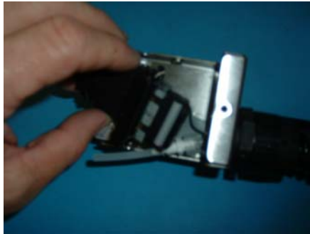
Figure 97: Pull Printhead Out
