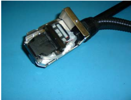
Figure 93: Remove Front and Side Covers
